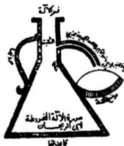
Fig.1. The Apparatus Used to Calculate Specific Gravity of Stones (Ansari, 1975)
